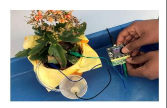
This device was created and used by BMS students to check soil composition and activate a water pump.
